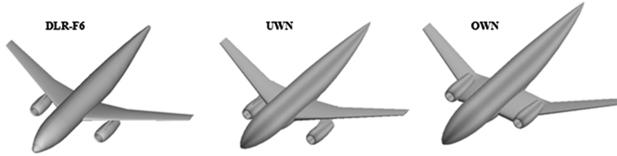
Fig. 2 Evolution of the UWN and OWN configurations from the DLR-F6 geometry.
